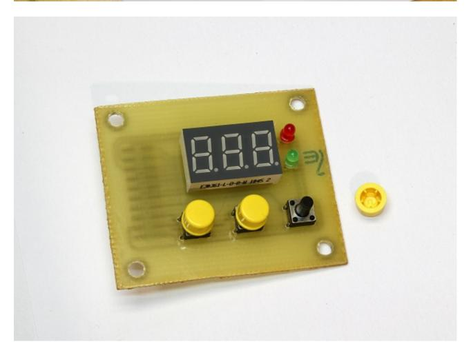
If your front panel is built around PCB, you need to adjust the height of PCB stands so that display(in this case) would be flush with FP surface. The front panel label should stick to the display, so that digits would show up through the label perfectly.
