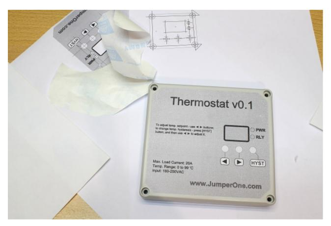
Now when label is in place, cut a piece of laminating sheet, aka cold laminating film(self-adhesive clear film) to the exact size of your front panel label.
